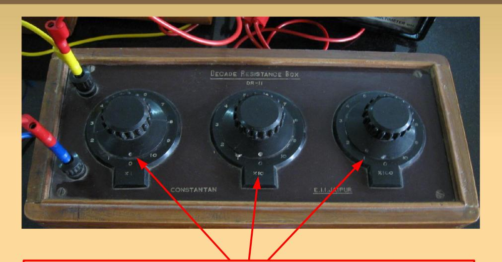
Dials of Resistance Box adjusted to 0, 0, 1: R = 0x1 + 0x10 + 1x100 = 100 ohm
